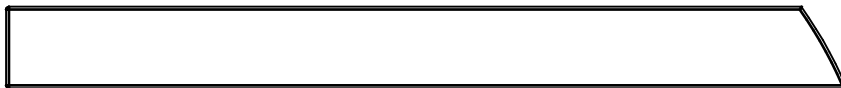
P17 - W100920 - Door Board - .625" x 3.375" x 35" (16mm x 86mm x 890mm) - Qty 1
