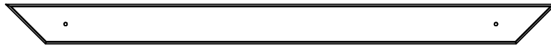
Q6 - W100914 - Sunburst Board - .625" x 2.375" x 32.875" (16mm x 60mm x 835mm) - Qty 2
