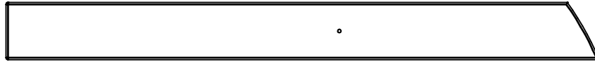
P16 - W100919 - Door Board - .625" x 3.375" x 35" (16mm x 86mm x 890mm) - Qty 1
