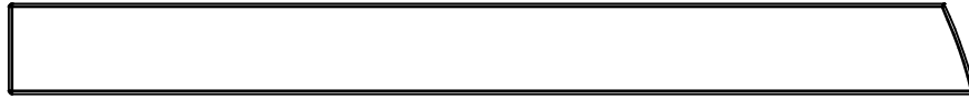
P15 - W100918 - Door Board - .625" x 3.375" x 36.25" (16mm x 86mm x 920mm) - Qty 2
