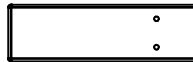
Q8 - W100916 - Sunburst Board - .625" x 2.375" x 7.875" (16mm x 60mm x 200mm) - Qty 4
